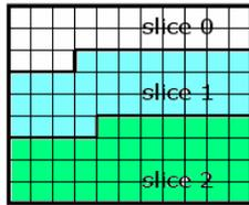
Fig. 5: Partition of a frame into slices using Arbitrary Slice Ordering (ASO).
