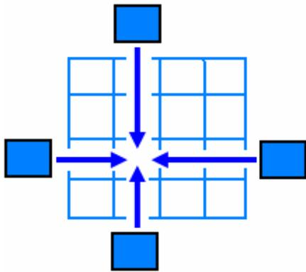
Fig. 7: Spatial Interpolation. The corrupted region is recovered from surrounding correctly decoded pixels.
