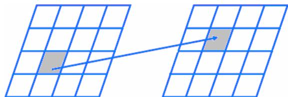
Fig. 9. Motion compensated temporal interpolation. The motion vector in conjunction with the transmitted DCT coefficients are used to achieve effective prediction of missing or corrupted blocks as motion compensated blocks are based on a previously decoded frame.
