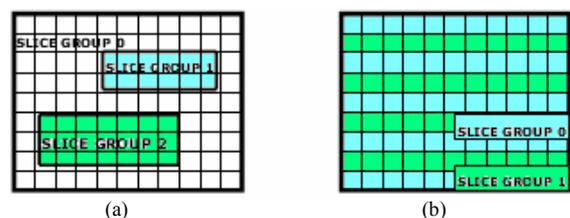
Fig. 4. Partition of a frame into slices using Flexible Macroblock Ordering (FMO). Two different partitions are given in (a) and (b).
