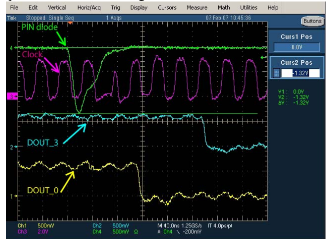
Fig. 5. Clock upset in the CLB shift register configuration
