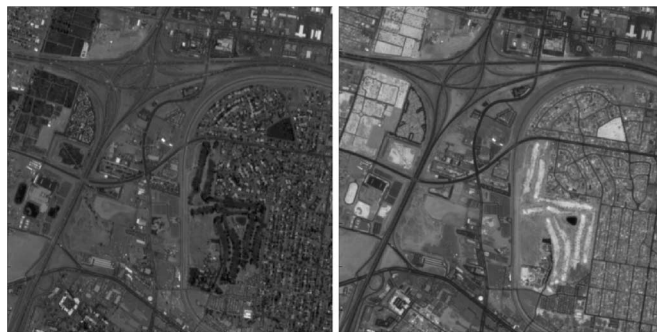
Fig. 10. Band A (0.485 \mu\text{m} ) and Band D (0.810 \mu\text{m} ) collected by the MTI satellite over Albuquerque, NM.
