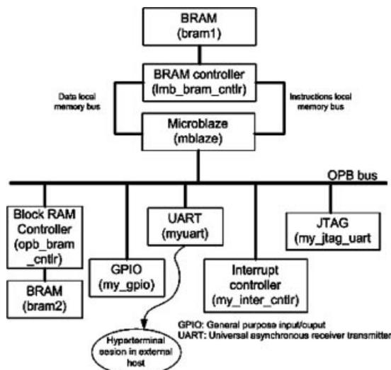
**Figure 5** Part of the testing phase included developing projects to use on the board (and to provide to other universities). This project (freely available online) is a virtual Microblaze microprocessor that was used to drive a HyperTerminal and an LED.
