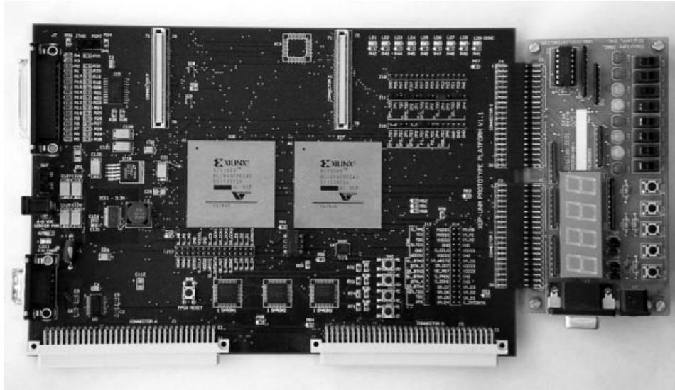
**Figure 1** The completed XUP-UNM platform with mated Digilent I/O board is shown here. By co-ordinating the design effort with the Digilent Corporation, interfacing with their series of peripheral input and output boards was accomplished. Their boards possess the capabilities including ADC, DAC, wire wrapping, and LCD.
