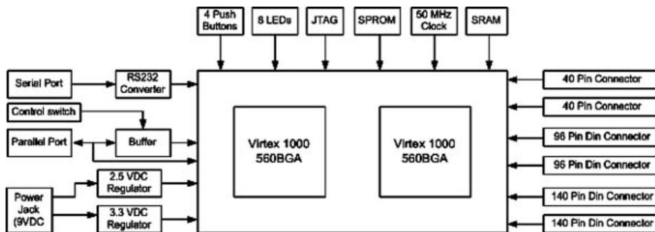
**Figure 2** During the design phase, a block diagram of all major components was created. This allowed for a more complete requirements analysis. This diagram was presented to students and instructors for feedback to ensure a variety of needs were addressed.
