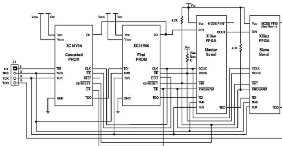
**Figure 3** Dual FPGA on a single platform greatly increases the project possibilities available to students. An inexpensive dual FPGA PCB is unavailable from major student platform providers. The interfacing between the cascaded PROMs and the dual FPGA devices was unique and required strict adherence to Xilinx specifications (Courtesy Xilinx Corporation).
